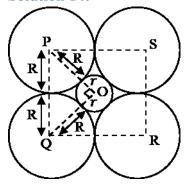
A sphere with centre O, is fitted into the octahedral void as shown in the above figure. It can be observed from the figure that  $\triangle$  POQ is right-angled
