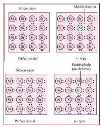
**p-type semiconductor:** The semiconductor whose increased in conductivity is a result of electoron hole is called a p-type semiconductor. When a crystal of group 14 elements such as Si or Ge is doped with a group 13 element such as B, Al, or Ga (Which contains only three valence electrons), a p-type of semiconductor is generated.
